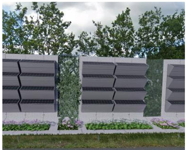
2 rows of ZigZagSolar cassettes with transparent sections and vegetation in between.
